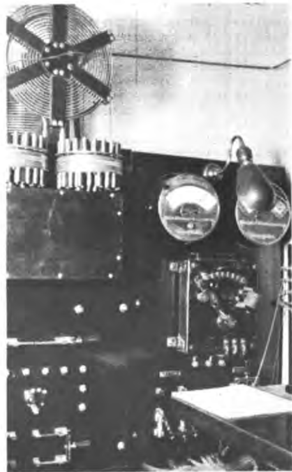
TRANSMITTER SET ON THE SS STARR 'WPS'. KILBOURNE & CLARKE 60 CYCLE SET UP OF 1915 VINTAGE.
